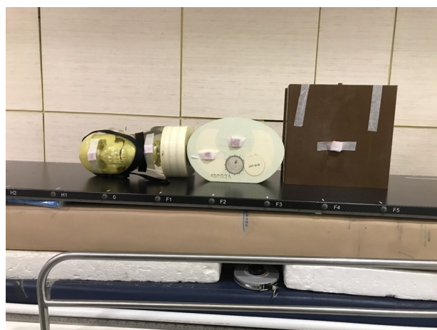
Figure 3. TBI phantom for mid-plane dosimetry.
