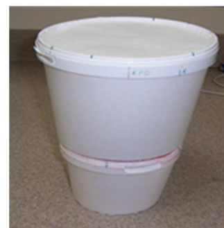
Figure 2. Two can phantoms with lid kept one over the other simulate the regions above and below the knee in terms of variations in thickness, as well as tapering effect. The bottom side of the top can and top side of the bottom can filled with 8 mm thickness of dental wax, to provide smooth surface as well as no air gap for keeping a film in between. Water is filled in the two cans to provide scattering conditions similar to leg.
