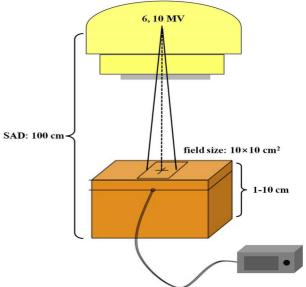
**Figure 2.** The distance between the ray source and the center of the ion chamber was fixed at a SAD of 100 cm. The field size was 10x10 cm<sup>2</sup> and the radiation energies of the photon rays were 6 MV and 15 MV.
