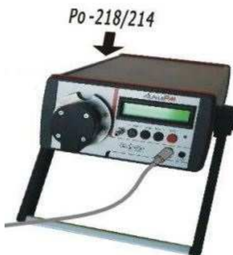
Figure 1. Typical alpha progeny meter (Saphymo GmbH).
