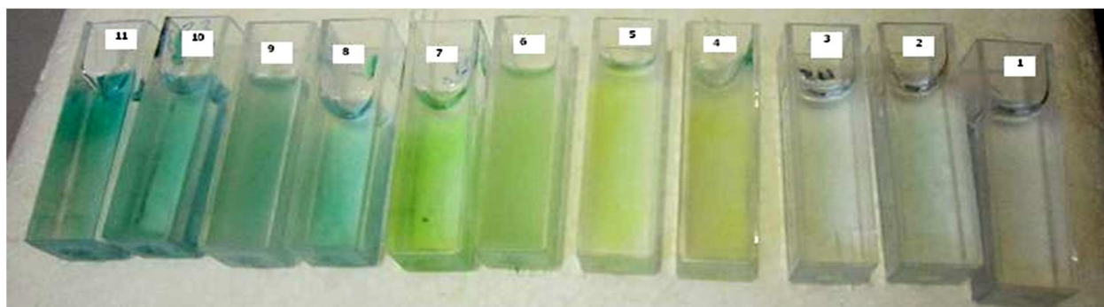
Figure 5. PRESAGE filled cuvettes with and without NPs at dose of 10Gy. 1) PRESAGE without NPs. 2) PRESAGE with 20µg/ml ZnO NPs. 3) PRESAGE with 20µg/ml ZnO NPs doped with %5 Gd. 4) PRESAGE with 500µg/ml ZnO NPs. 5) PRESAGE with 500µg/ml ZnO NPs doped with %5 Gd. 6) PRESAGE with 1000µg/ml ZnO NPs. 7) PRESAGE with 1000µg/ml ZnO NPs doped with %5 Gd. 8) PRESAGE with 3000µg/ml ZnO NPs. 9) PRESAGE with 3000µg/ml ZnO NPs doped with %5 Gd. 10) PRESAGE with 4000µg/ml ZnO NPs. 11) PRESAGE with 4000µg/ml ZnO NPs doped with %5 Gd.
