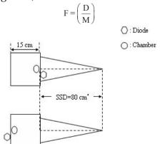
**Figure 1.** Determination of the entrance and exit calibration factors for diodes. The diodes were calibrated in reference condition: 80 cm SSD, 10×10 cm field size, temperature=25 C, gantry angle=90, 15 cm Perspex water phantom.
