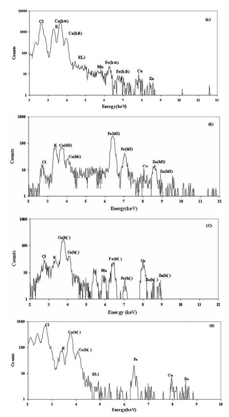
**Figure 1.** Typical spectra for PIXE analysis of: (a) bile, (b) gallbladder, (c) gallstones (center), and (d) gallstones (shell). A 175 m Maylar filter are used in front of detector.
