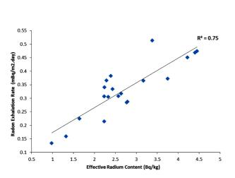
**Figure 2.** Correlation between the effective radium content and radon exhalation Rate in samples under study.
