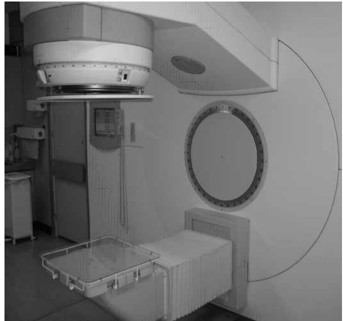
Figure 2. The Cablon Theraview EPID attached to an Elekta SL15 linear accelerator.
