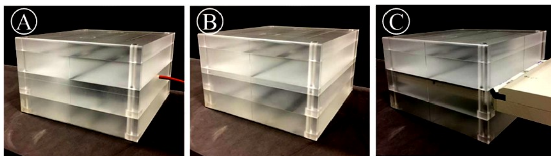
Figure 1. A multi-purpose phantom using (A) the ionization chamber, (B) the EBT3 film, and (C) the MapCHECK system.
