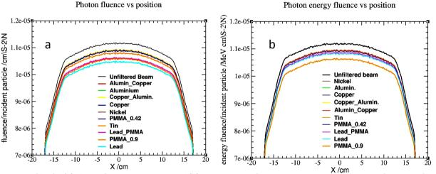
**Figure 2.** Profiles for **(a)** Photon fluence vs. position and **(b)** Photon energy fluence vs. position along the x-axis for various filters and without filter at treatment distance of 80 cm from the source.
