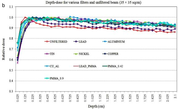
Figure 5. Depth-dose distributions for various filters and unfiltered beams for  $35 \times 35$  cm<sup>2</sup> field size (a) for only due to photons in the beam and (b) due to all particles photon, electron and positron in the beam.
