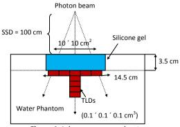
Figure 1. Inhomogeneous phantom.
