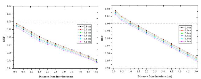
Figure 3. Dose enhancement factor for varies silicone gel thickness as a function of distance for the 6 MV photon beam with  $10 \times 10 \text{ cm}^2$  field size.
