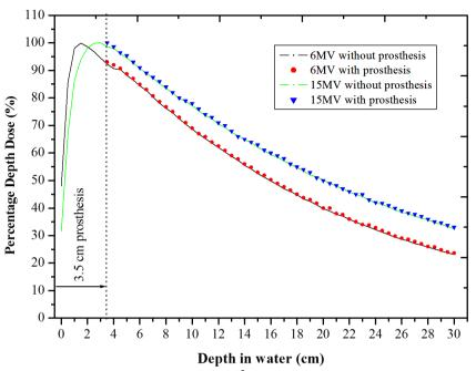
Figure 2. Percentage depth dose distribution curves for  $10 \times 10$  cm<sup>2</sup> field size, calculated with and without the silicone gel breast prosthesis for 6 and 15 MV photon beams.
