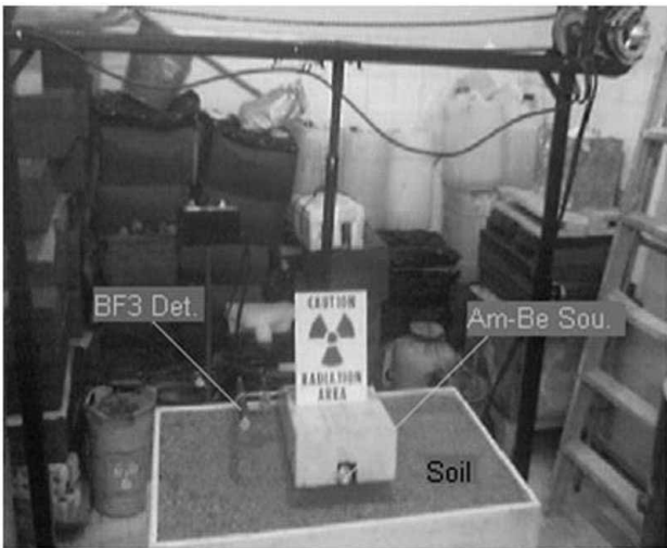
Figure 5. Photograph of landmine detection set-up.
