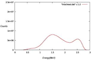
Figure 3. Resultant photoneutron spectrum.
