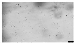
Figure 2. Tracts in etched film after irradiation.
