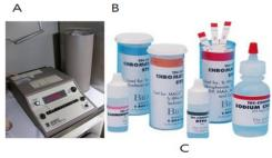
Figure 1. Dose calibrator and materials for testing: (A) dose calibrator, (B) cylinder tube and vial, (C) developing solvent.
