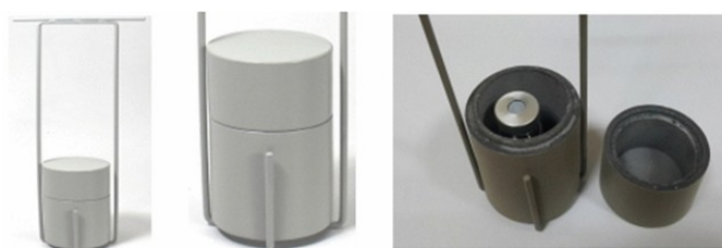
Figure 2. Moly-Shield used for the radionuclide purity measurement.
