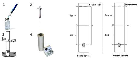
**Figure3.** Four steps: **(1)** place solvent intro developing vial; **(2)** spot ratiolphamaceuticals on chromatography strip; **(3)** develop strip in solvent; **(4)** count the strip using a well detector, dose calibrator or radio-chromatogram scanner, for measuring RCP using the thin-layer-chromatography double-solvent method, showing control kits and solvents.
