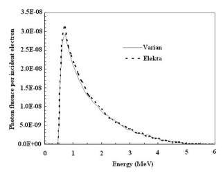
Figure 7. Contamination electron energy spectra for Elekta and Varian linacs on phantom surface for field size of 20×20 cm<sup>2</sup>.
