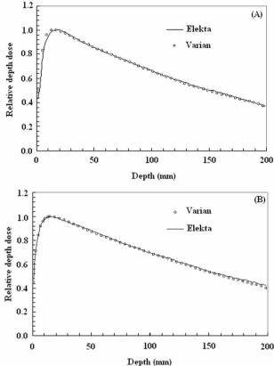
Figure 9. Relative depth dose curves for 6MV photon beams of Elekta and Varian linacs. (A) 10×10 cm<sup>2</sup> (B) 20×20 cm<sup>2</sup> field sizes.
