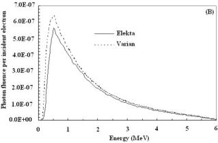
**Figure 6.** Photon energy spectra for 6MV photon beams of Varian and Elekta linacs for different field sizes. (A) 10×10 cm<sup>2</sup> (B) 20×20 cm<sup>2</sup>.
