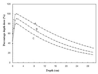
**Figure 2.** Percent depth dose curves of 6 MV beam of Elekta linac for different field sizes (A) 30×30 cm<sup>2</sup> (B) 10×10 cm<sup>2</sup> (C) 5×5 cm<sup>2</sup>. The curves B and C were scaled to 0.9 and 0.8 to inclusion on the same graph.
