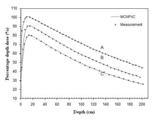
Figure 3. Percent depth dose curves of 6 MV beam of Varian linac for different field sizes (A) 30 ×30 cm<sup>2</sup> (B) 10×10 cm<sup>2</sup> (C) 5×5 cm<sup>2</sup>. The curves B and C were scaled to 0.9 and 0.8 to inclusion on the same graph.
