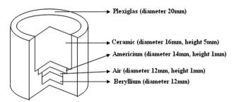
Figure 1. Designed Am-Be neutron source.
