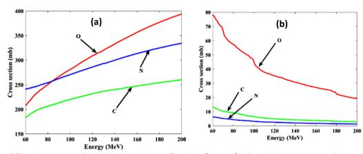
**Figure 4. (a)** Total neutron production cross-section as a function of energy for the incident proton on carbon, oxygen and nitrogen; **(b)** Total photon production cross-section as a function of energy for the incident proton on carbon, oxygen, and nitrogen.
