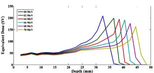
**Figure 2.** Depth dose profiles in the breast of ORNL-female phantom for 1nA incident proton with an energy range of 60-70 MeV on the left breast. A specific color demonstrates the results of each proton energy.
