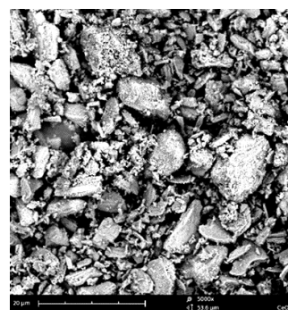
Figure 1. SEM image with 5000x magnification showing the size distribution of cerium oxide nanoparticles purchased from US Research Nanomaterials, Inc (Houston, USA).
