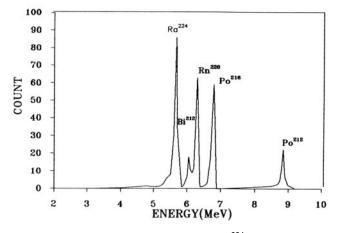
**Figure 3.** Alpha particle spectrum of <sup>224</sup>Ra microprecipitate on millipore filter.
