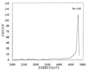
**Figure 2.** Alpha particle spectrum of <sup>226</sup>Ra microprecipitate on millipore filter immediately after preparation.
