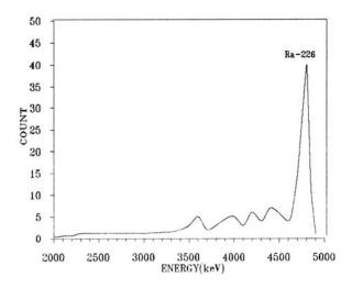
**Figure 1.** Alpha particle spectrum of <sup>226</sup>Ra microprecipitate on Whatman filter immediately after preparation.
