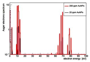
**Figure 4.** Auger-electrons spectrum resulting from proton beam energy of 200 MeV for 20 ppm and 200 ppm of AuNPs concentrations.
