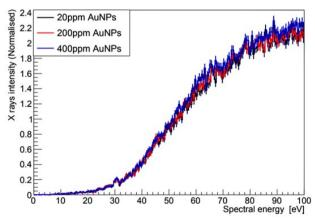
Figure 3. Spectrum of secondary X-rays from proton beam energy of 200 MeV for 20 ppm (respectively 200 ppm and 400 ppm) concentrations.
