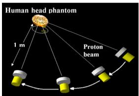
**Figure 1.** Simulation of proton therapy of a tumor inside a head using a rotary accelerator with a monoenergetic proton beam of 200 MeV.
