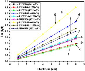
Figure 3. Ln (IO/I) against thicknesses for the phthalonitrile/ WB samples at Cs-137 and Co-60 energy sources.
