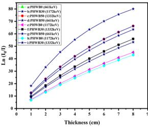
**Figure 5.** The radiation protection efficiency as the function of phthalonitrile/WB composites' thickness different energies.
