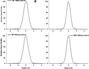
Figure 9. Dose profile symmetry with mirror removal in field at MeV (A) 6 and (B) 9 MeV energies.
