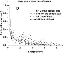
Figure 8. The photon and electron energy flux reached to phantom surface on the central axis and different off-axis distances at SSD =100 cm. For  $0.25 \times 0.25$  cm2 field (A), (B) at energy 6 MeV, (C), (D) at energy 9 MeV.
