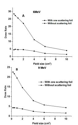
Figure 4. Dose ratio for PSFF and SFF modes; (A) 6 MeV, (B) 9 MeV.
