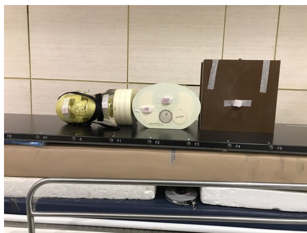
Figure 3. TBI phantom for mid-plane dosimetry.
