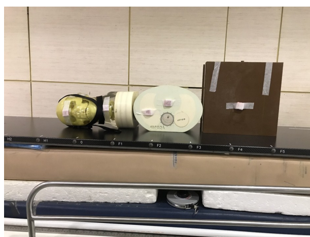
Figure 3. TBI phantom for mid-plane dosimetry.
