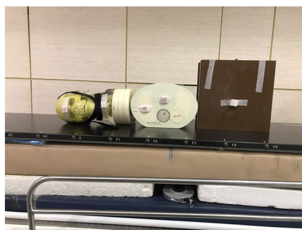
Figure 3. TBI phantom for mid-plane dosimetry.
