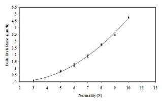
**Figure 2.** The bulk etching rate variation versus normality of an aqueous solution of NaOH (at Temperature: 70°C for Time: 6h)
