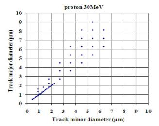
Figure 6. Major track diameters versus minor track diameters Ep =30 MeV.
