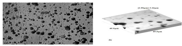
Figure 5. The typical etched tracks registered by CR-39 detector viewed by; a) optical microscope; b) atomic force microscope.
