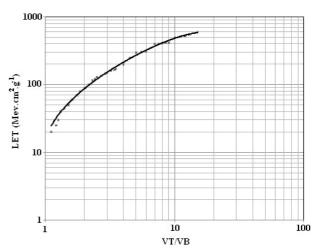
Figure 1. The obtained calibration curve from irradiations of <sup>12</sup>C to <sup>56</sup>Fe ions, with LET in water ranging from 7.9 to 200 keV/µm.
