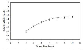
Figure 4. The bulk etching rate dependency of CR-39 versus etching time (6N NaOH at 70  $^{\circ}$ C).
