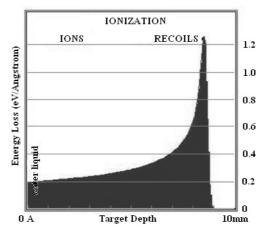
Figure 11. Depth dose distribution of the 30 MeV proton beam.
