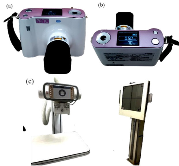
Figure 1. X-ray devices used in the experiment (a) handheld X-ray device front view, (b) handheld X-ray device upper view, (c) stationary X-ray device.
