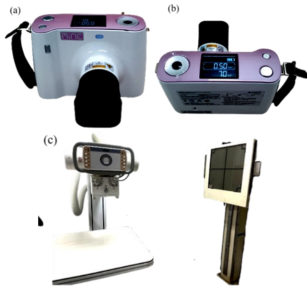
Figure 1. X-ray devices used in the experiment (a) handheld X-ray device front view, (b) handheld X-ray device upper view, (c) stationary X-ray device.
