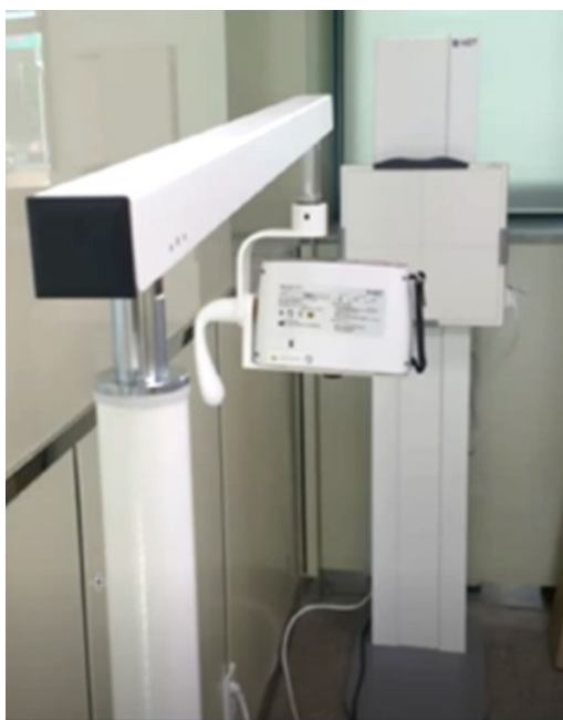
Figure 2. A detector stands capable of holding the detector and a tripod capable of holding the handheld X-ray device.
