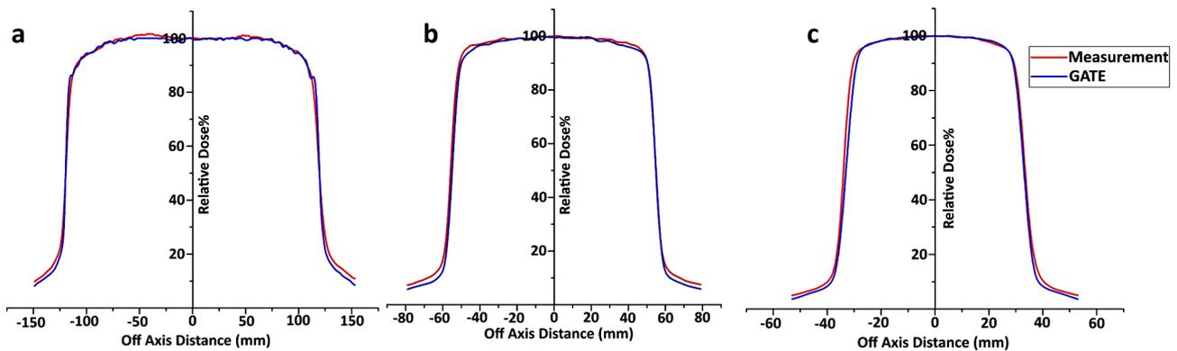
**Figure 4.** Comparison of transverse profiles between GATE simulations and measurements in (a) 6 × 6 cm<sup>2</sup>, (b) 10 × 10 cm<sup>2</sup>, and (c) 20 × 20 cm<sup>2</sup> field sizes.
