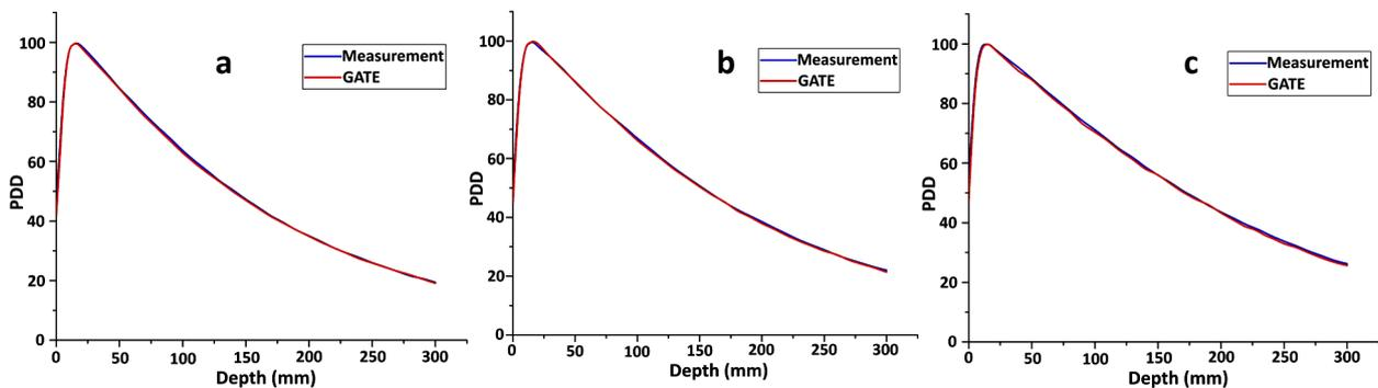
**Figure 3.** Comparison of percent depth dose (PDDs) between GATE simulations and measurements in (a)  $6 \times 6$  cm<sup>2</sup> (b)  $10 \times 10$  cm<sup>2</sup>, and (c)  $20 \times 20$  cm<sup>2</sup> field sizes.
