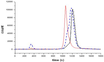
Figure 2. RP-HPLC analysis after labeling with 99mTc for kit A (dot); kit B (solid) and kit C (dash dot).
