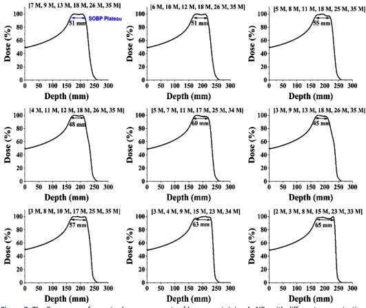
Figure 7. The Bragg curve for sextuple arrangements of layers containing AuNPs with different concentrations.
