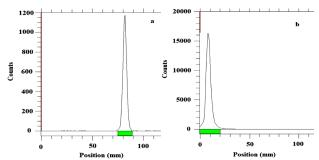
Figure 1. RTLC chromatogram of 177Lu (a) and 177Lu-DTPA-CHX-Cetuximab-PAMAM (b) at 60 min after preparation using the mobile phase of 0.1 M citrate buffer (pH 5), and the stationary phase of Whatman No. 1 paper.
