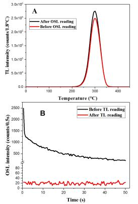
**Figure 4.** OSL and TL reading modes combination. **A)** Effect of OSL firstly readied on TL glow curve and intensity. **B)** Effect of TL firstly readied on OSL signal.
