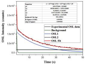
**Figure 2.** 2 Gy OSL curve decomposition into fast (OSL1) and slowly (OSL2) decaying types components. The data represent the fit of experimental signal by the proposed model. Model and fit function accuracy is evaluated using square root of the reduced Chi-squared (Chi-sqr) test.
