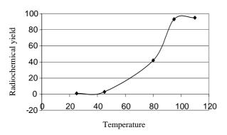
**Figure 5.** Effect of temperature on radiochemical yield of [<sup>62</sup>Zn] BLM at optimized conditions.
