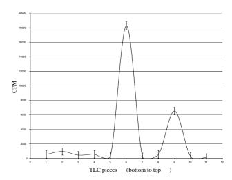
**Figure 2.** Radio chromatogram of a [<sup>62</sup>Zn] BLM sample at optimized condition.
