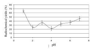
**Figure 3.** Effect of pH on radiochemical yield of [<sup>62</sup>Zn] BLM at 80°C.
