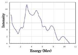
Figure 1. The neutron energy spectrum of Am-Be source.
