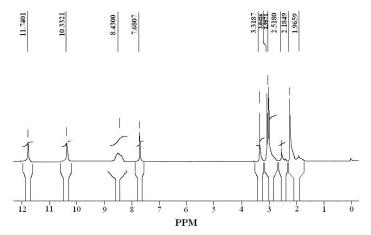
**Figure 6.** <sup>1</sup>H-NMR spectrum of pure PTSM used in the labeling procedure.
