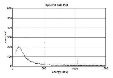
**Figure 7.** Gamma spectroscopic diagram of the final purified [<sup>64</sup>Cu] CuCl<sub>2</sub> solution.
