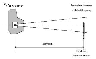
**Figure 2.** Reference conditions for calibration in terms of air kerma for <sup>60</sup>Co gamma radiation.
