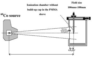
**Figure 3.** Reference conditions for calibration in terms of absorbed dose to water for <sup>60</sup>Co gamma radiation.
