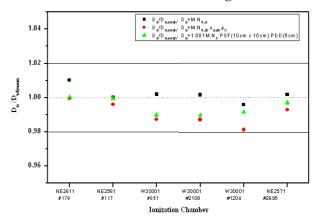
Figure 4. Results of absorbed dose rate Variation at a reference point in a <sup>60</sup>Co radiotherapy beam as determined by three formalisms using IAEA calibrated chambers. The reference point was located on the central axis of the beam, at 5 cm depth in a 30 cm × 30 cm × 30 cm water phantom. The distance from the source to the phantom surface was 80 cm and the field size at this distance was 10cm × 10cm.
