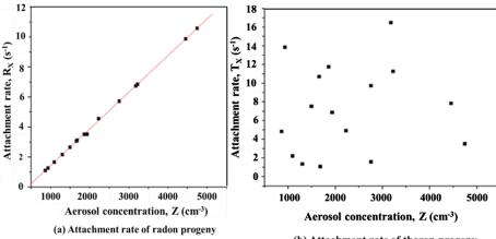
Figure 3. (a) Variation of aerosol concentration (Z) and radon progeny attachment rates (RX) and (b) variation of aerosol concentration (Z) and thoron progeny (TX).
