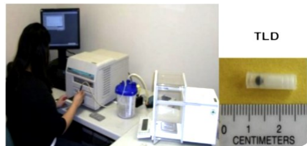
Figure 15. The remote dosimetry audit with thermoluminescent dosimeters-TLDs in IROC-Houston (34).
