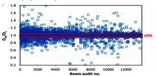
**Figure 13.** Results of a dosimetry audit conducted by the IAEA/WHO in 1969-2018. 13,756 audits of photon beams generated by 4,427 radiotherapy devices in 2,364 radiotherapy centers from 136 IAEA member states <sup>(31)</sup>.
