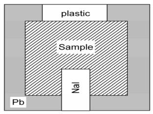
Figure 2. Source-detector geometry.  $\beta$  and  $\gamma$  radiations are emitted from voluminous sample and are detected by plastic and Nal scintillators, respectively.
