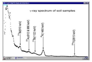
Figure 3. A  $\gamma$ -ray spectrum of a soil sample measured by using NaI(TI) scintillator.
