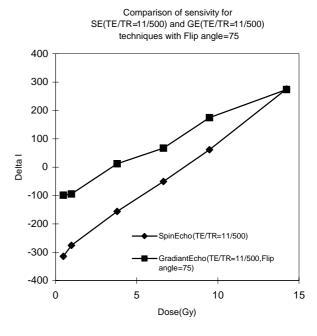
**Figure 3.**  $\Delta$ I profiles for dose range of 0.47 to 14.23 Gy, 1) SE technique with TE=11,TR=500 and 2) GRE technique with TE=11,TR=500 and flip angle 75. The sensitivity in (SE) is 39.9 Gy<sup>-1</sup> while for (GRE) is 26.9 Gy<sup>-1</sup>.
