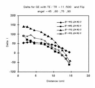
**Figure 5.** Curves obtained with GRE technique for TE=11ms, TR=500ms with flip angles of  $45^{\circ}$ ,  $60^{\circ}$ ,  $75^{\circ}$ , and  $90^{\circ}$ . phantoms were Plexiglas irradiated to a certain dose.
