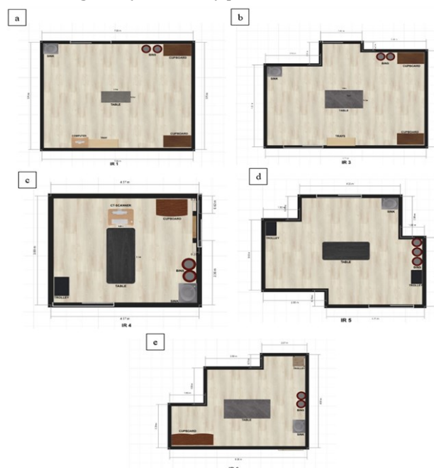
Figure 1. Geometries of angiography rooms for simulation (a) IR1, (b) IR3, (c) IR4, (d) IR5, (e) IR6. The geometries represent different interventional radiology suites within the clinical setting, each with unique room dimensions. These room geometries were modelled based on actual floor plans and equipment layouts to accurately reflect clinical practice and ensure realistic dose estimation using the Monte Carlo GATE simulation framework. (IR 1 (5.75 x 7.00) m, IR 3 (4.55 x 7.70) m, IR 4 (3.89 x 4.57) m, IR 5 (3.43 x 5.76) m, IR 6 (4.22 x 4.65) m measurement).
