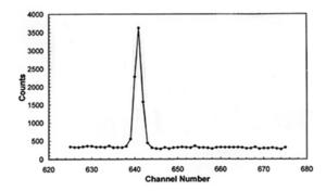
**Figure 1.** Spectrum of <sup>7</sup>Be in surface air.
