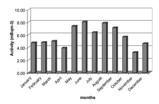
**Figure 3.** Monthly variations in the concentrations of <sup>7</sup>Be in the surface air in Tehran station during 2002.
